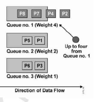
Some implementations of the WRR algorithm provide prioritization by dispatching a configurable number of bytes each round rather than a number of packets. The Cisco custom queuing (CQ) mechanism is an example of this implementation.
