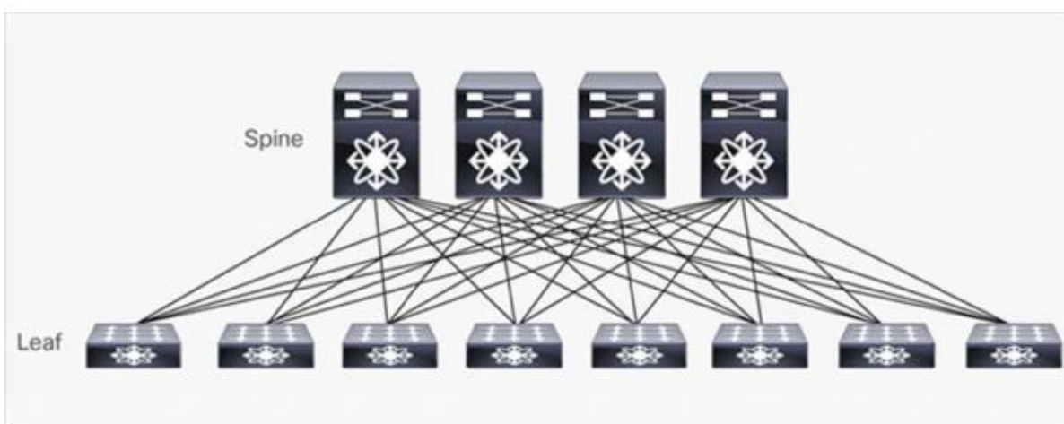
Figure 31-12 Typical spine-and-leaf topology
